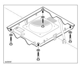
■ Screw the mounting plate through the ceiling and into the structural framing using 8 x 60 lag bolts and washers. Once tight, make sure that the mounting plate can safely support the weight of the hood.
